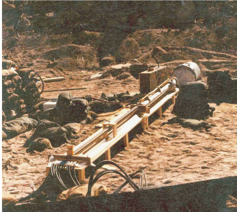
Fig. 30. Strip generator powered railgun at Ancho Canyon firing site (LANL).
