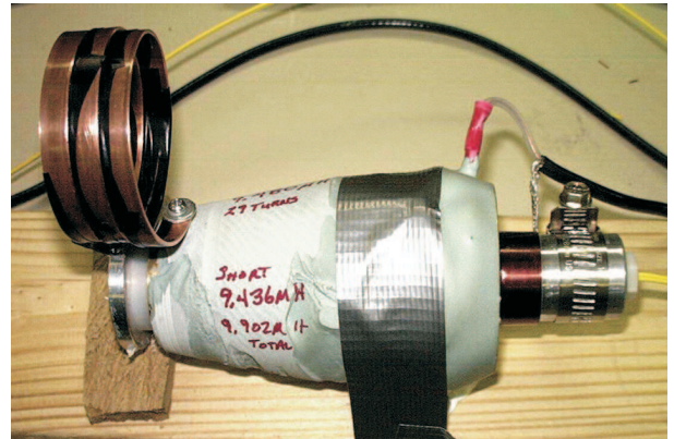
Fig. 35. Texas A&M 25 mm diameter FCG (Courtesy of Dr. B.L. Freeman, Texas A&M University.)
